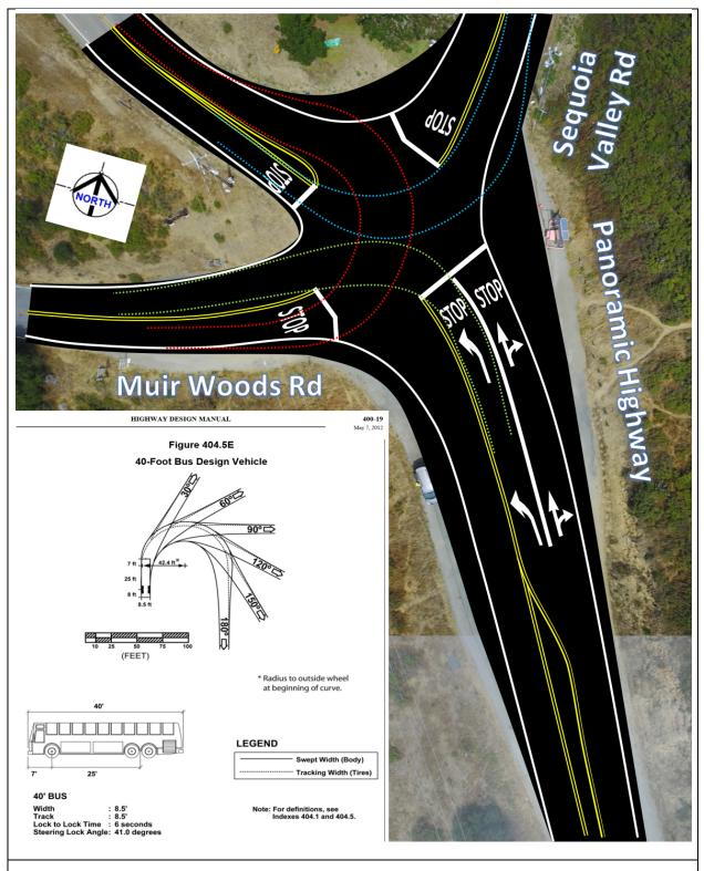
Figure 11. Alt. 4 Bus Design Vehicle Turn Check for Left Turns: Ample Space.
