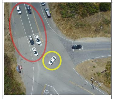
3. The vehicle in the yellow circle is causing 5 cars to stop who have the right-of-way. The 5 cars with the right-of-way are not progressing forward into through lane north on Panoramic Highway.
