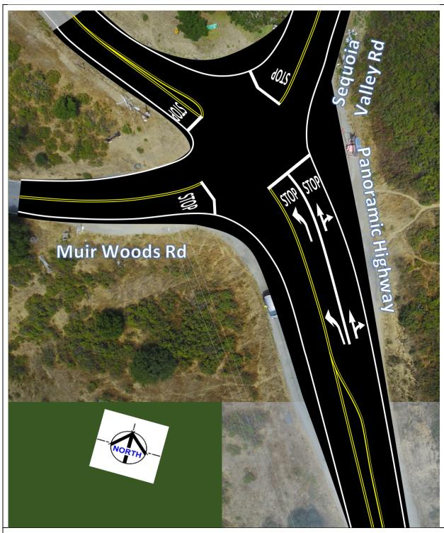
Figure 10. Alt. 4 Intersection Layout, Striping and Pavement Markings
