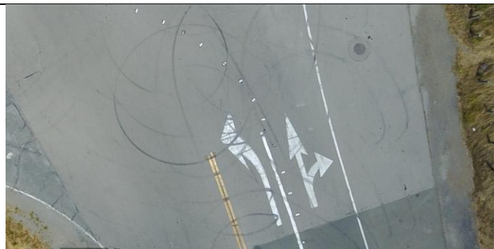
Pavement Marking details for northbound approach, Panoramic Highway. Raised Markers for left turn lane guidance to Muir Woods Road. Left Turn lane separate from Through/Right lane. No stop. LT lane is only 10 feet wide. Thru/RT lane is 11.5 feet wide, as measured in field.
